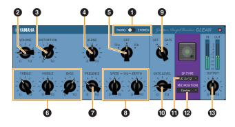
This amp type is optimized for clean tones, effectively simulating the tight brilliance of transistor amplifiers. The tonal character of this amp model provides an ideal platform for recording with multi-effects. It also features built-in chorus and vibrato effects.
