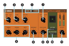
The LEAD amp type simulates a high-gain tube amp that is rich in overtones. It is ideally suited to playing lead guitar lines that will project well in an ensemble, but it can also be set up for crisp accompaniment tones as well.
