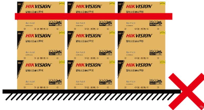
Figure 20. Avoid Stacking Three or Higher During Storage
