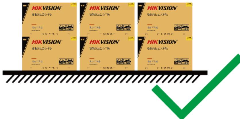
Figure 19. Stacking in at Most Two Layers During Storage
