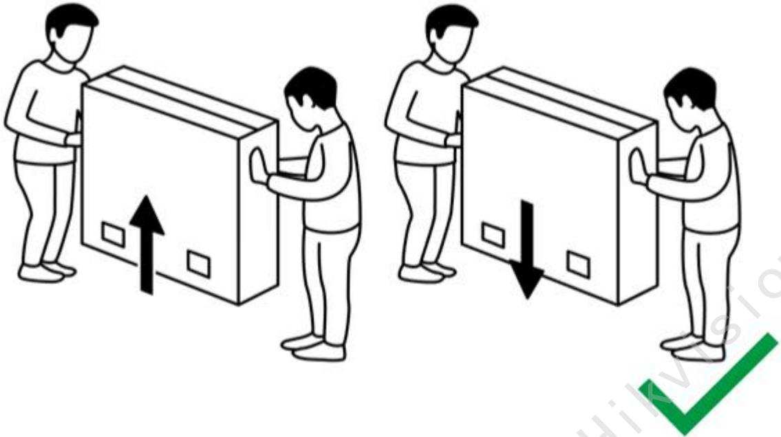
Figure 16. Two Workers Lifting and Lowering a Package Box Simultaneously
