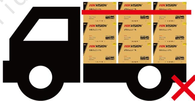
Figure 5. Avoid Stacking Three or Higher During Transportation
