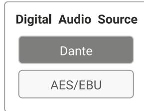
When Dante™ is selected, the four Dante™ channels are available on E/F/G/H inputs. When AES/EBU is selected, the two AES/EBU channels (from the XLR input) are available on E/F inputs, G/H inputs being unused.
