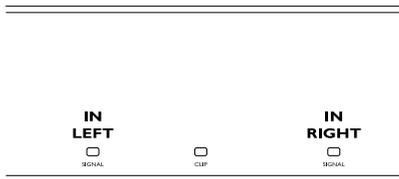
A center red clip LED will inform the user that at least one analog input of the controller is clipping: reduce then audio source level to prevent distortion.
