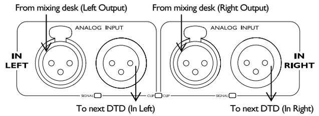
AES/EBU signal can be connected to the back panel female XLR3 input.
