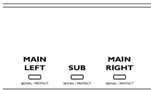
On each output a yellow signal LED will light if the controller is limiting its output to protect the speaker.
