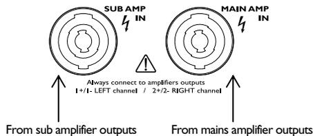
**WARNING!** Use at least a 2.5 mm<sup>2</sup> (AWG #13) double insulated cable.
