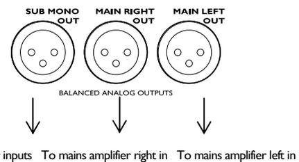
On the DTD-I, use the back panel terminal block connectors to connect the balanced analog output signal to the amplifier inputs.
