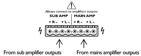
**WARNING!** Use at least a 0.5 mm<sup>2</sup> (AWG #20) double insulated cable.
