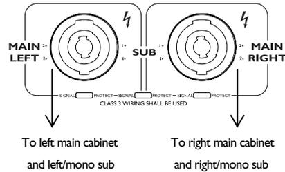
On the DTD-I, use a four wire speaker cable to connect the output of the amplifiers to the back panel terminal block connectors.
