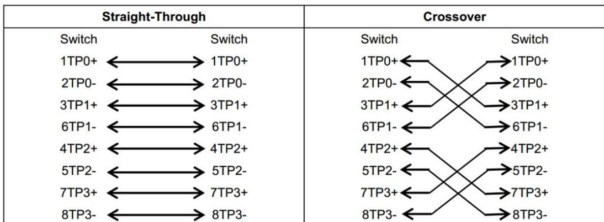
10BASE-T uses Category 3, 4, 5, 5 100-ohm UTP/STP and 1000BASE-T uses Category 5 100-ohm UTP/STP for connections. Both support a maximum length of 100 meters. The following table shows 100BASE-TX/10BASE-T pin assignments.
