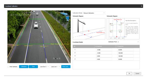
Figure 3-2 Manual Calibration
