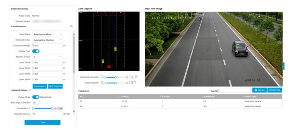
Figure 3-1 Set Radar Parameters
