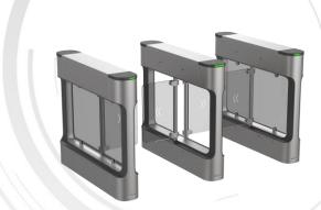
The DS-K3B411BX series swing barrier with 6 pairs of IR lights is designed to detect unauthorized entrance or exit. By adopting the swing barrier integratedly with the access control system, person should authenticate to pass through the lane via presenting IC or ID card, scanning QR code, etc. It is widely used in attractions, stadiums, construction sites, residences, etc.
