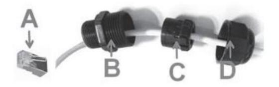
(3) After threading the network cable through the cable gland assembly, install an RJ-45 connector on the unterminated end of the network cable. Wrap waterproof materials around the network cable between B (split gasket) and C (grommet).
