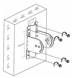
(3) Install the AP on the mounting plate to the mounting bracket. Use four M6 screws to join the mounting plate and the bracket. Adjust the orientation of the AP before tightening the screws.
