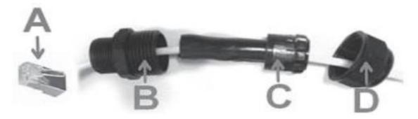
(4) Insert the RJ45 connector into the Ethernet/PoE port of the access point, and tighten the cable gland assembly in sequence of part B, C and D to complete the installation.
