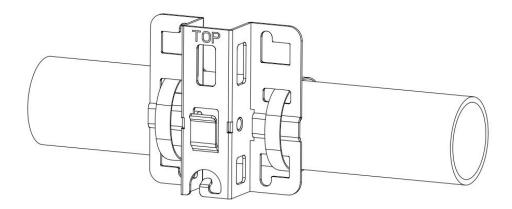
(3) Position the mounting arm on the mounting bracket with its two holes aligned to the screw holes on the mounting bracket.
