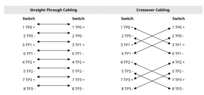
100BASE-TX/10BASE-T port can also be connected by cables of the preceding specifications. Besides, the 10BASE-T port can be connected by 100-ohm Category 3, Category 4, and Category 5 cables with a maximum distance of 100 meters (328.08 feet). 100BASE-TX port can be connected by 100-ohm Category 5 cables with a maximum distance of 100 meters (328.08 feet). The following figure lists definitions of pin signals for the 100BASE-TX/10BASE-T port.
