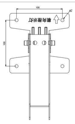
• For the pole-mounted access point, the pole diameter should meet the specified requirement.
