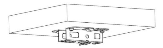
(2) Loosen the two M6 screws on the mounting plate assembly to remove the mounting arm. Rotate the mounting arm by 90 degrees clockwise until it is upright. Tighten two M6 screws to secure the mounting arm to the mounting plate.
