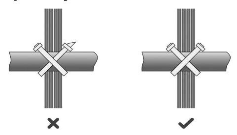
o When cables need to be bent, bind them first but do not tie cable ties within the bend. Otherwise, considerable stress may be generated in cables, breaking cable cores, as shown in <u>Figure 7-6</u>.
