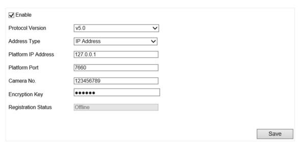
Figure 6-2 Connect to ISUP Platform
