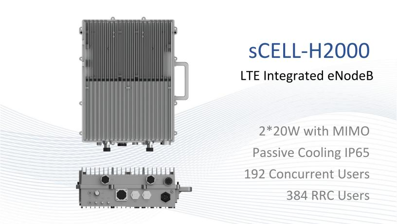
The sCELL-H2000 from SUNWAVE is an advanced outdoor LTE compact product that operates in TDD mode. This eNB provides users with high-speed broadband wireless access to the Internet using 2x20W output power (2x2 MIMO with 20W output each channel). This eNodeB can operate in 5, 10, 15 or 20 MHz bandwidth, supporting 192 concurrent users and 384 RRC users.
