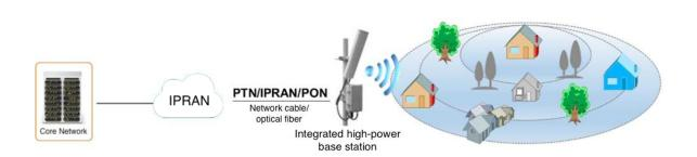
In rural and suburban areas, the wireless network coverage is relatively wide, but the users are less fixed than the fixed ones. By deploying LTE integrated high-power base stations in a town or natural village, the signal coverage in a small area can be achieved, reaching low Investment in rural 4G wireless access.
