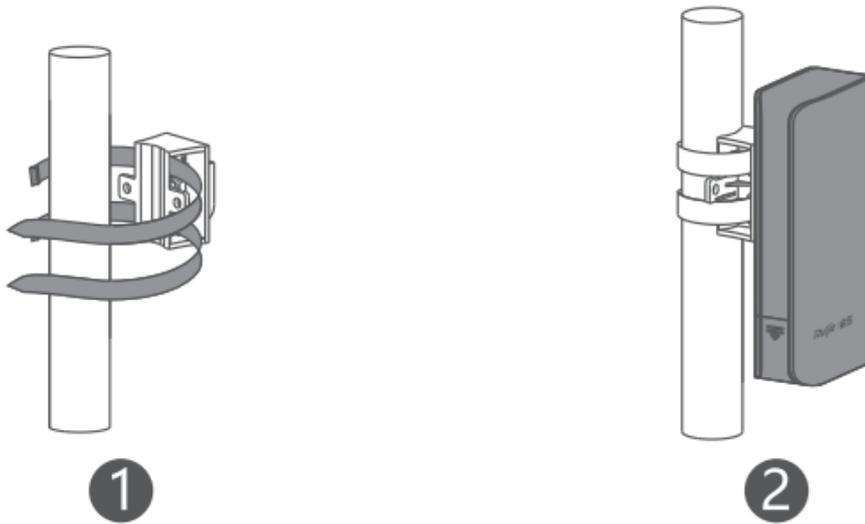
1. Secure the mounting bracket to the pole by threading two clamps through the mounting bracket.
