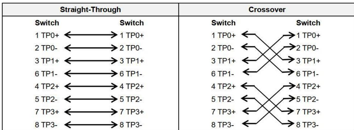
10BASE-T uses Category 3, 4, 5 100-ohm UTP/STP and 1000BASE-T uses Category 5 100-ohm UTP/STP for connections. Both support a maximum length of 100 meters. Figure 7-2 shows 100BASE-TX/10BASE-T pin assignments.
