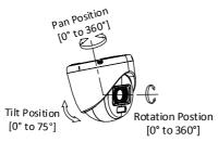
Figure 2-15 3-Axis Adjustment
