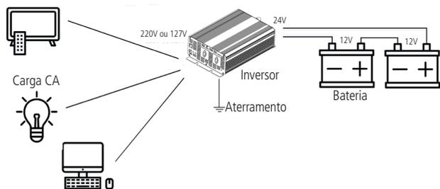
Antes de realizar as conexões desligue o interruptor Liga/Desliga do inversor
