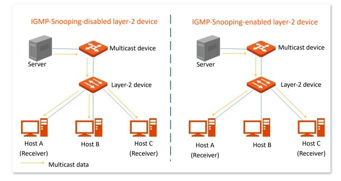
IGMP snooping only forwards data to the specific receivers through the layer-2 multicast, providing the following advantages:
