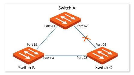
After calculation, switch A is selected as the root bridge, and the link between ports A2 and C6 is blocked.
