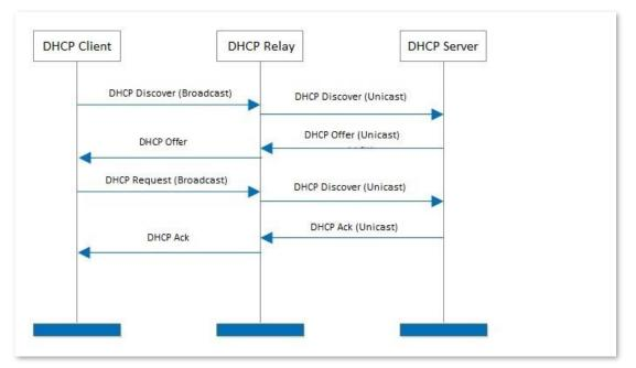
The working principles of DHCP Relay are shown below.
