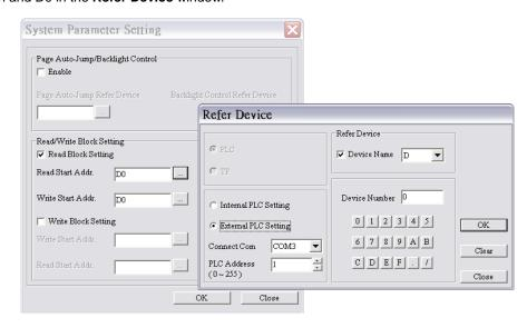
• Write Block Setting: The values in D10~D17 in TP70P are written to D10~D17 in the DVP series PLC.
