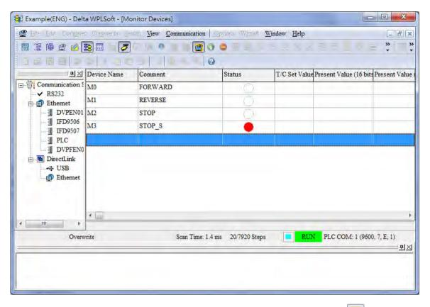
The states of the devices broght into the device monitoring table will be shown only if [ is pressed. If the users want to change the state of a device, they can right-click the device, and click an item on the context menu which appears. Mo is set to ON here. When Mo is ON, Yo is ON, the AC motor drive used rotates forwards, and the users can see that the forward rotation indicator on the screen of TP70P is green.
