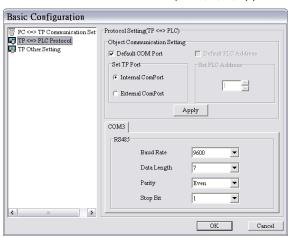
**Step 4:** Compile the program created, and download the program to TP70P. Connect COM3 on TP70P to an RS-485 communication port on a PLC.
