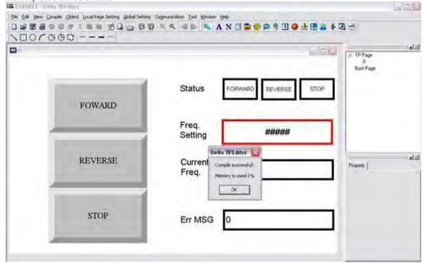
After the program is compiled, the users can download the program. After the users click **Write to TP** on the **Communication** menu, or on the standard toolbar, the **Download Setting** window will appear.
