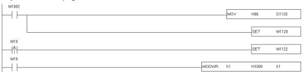
Step 6: When M10 is ON, users can see that the value displayed on the screen of TP70P is changed to 1.
