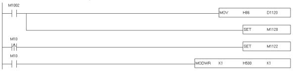
**Step 2:** Connect COM2 on TP70P-16TP1R to the two RS-485 wires connected to a DVP series PLC. When M10 is ON, Y0 on the DVP series PLC is ON.
