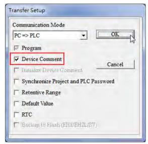
After the users select the **Device Comment** checkbox, the **System Block** window will appear. The users can select devices and set device ranges.
