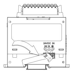
2. Use screws to secure the baffle.
