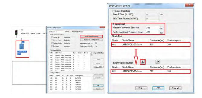
Click OK to confirm the setting. Download the parameters to the PLC. And then PLC can control the input/output of the IO module remotely.
