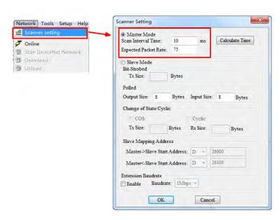
The explanation of Scan Interval Time and Expected Packet Rate is shown in the following table.
