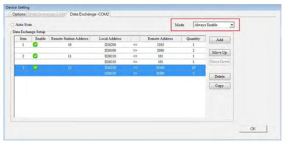
NOTE: If the Data Exchange Mode Control is set by the program, you can check and control the register address on the Normal Exchange Area page.
