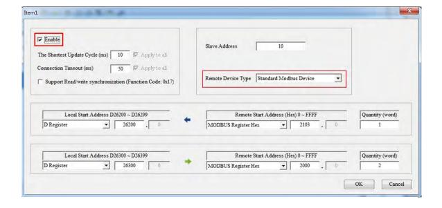
Select Standard Modbus Device as the Remote Device Type, enter the ASDA parameters, and check Enable.
