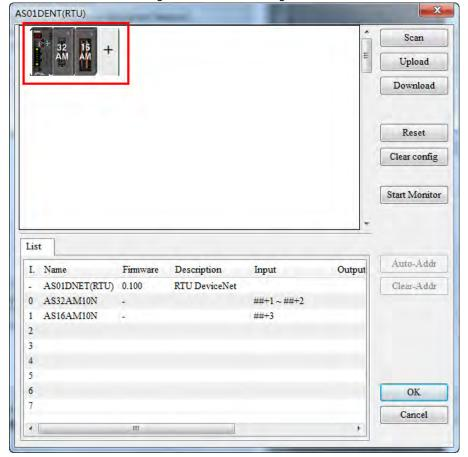
Double click **AS01DNET (RTU)** icon on the far left of the configuration page. Then the parameter setting interface of AS01DNET (RTU) comes out for setting the error handling method as follows.
