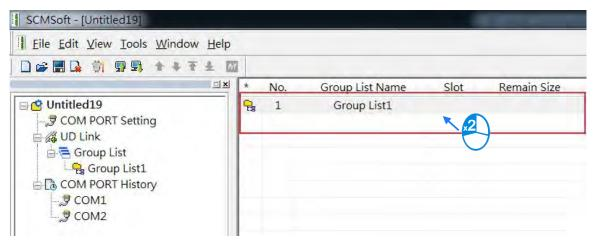
Give the group list a Name (this example uses "Slave\_Simulation") and select 1 (COM1) as the **Slot** number.
