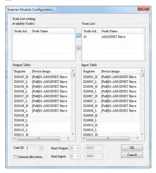
Click OK to finish the configuration above. Then download the configuration data to AS01DNET-A. During the download, the Warning dialog box will pop out if AS PLC is in RUN mode. Click OK to continue the download.
