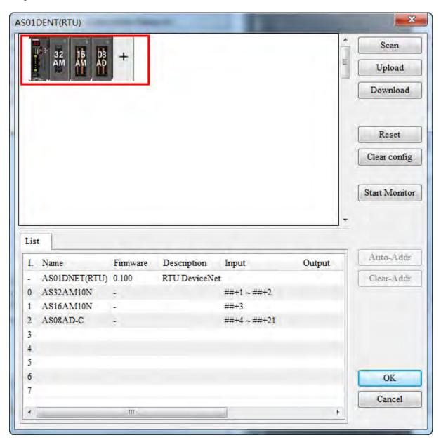
Double click the 08AD icon. Then the AS08AD-C configuration interface appears as below for configuration of parameter mapping of AS08AD-C module.
