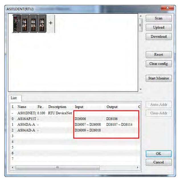
The software automatically assigns mapping addresses of module parameters in the arrangement order of modules connected to the right side of AS01DNET (RTU) from left to right.
