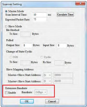
7. Click **Network** >> **Download** to download the extension baud rate setting to the master. After the download is completed, switch DR0 and DR1 of AS01DNET-A to ON. Finally, repower AS01DNET-A.
