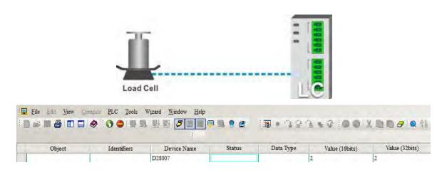
Step 8: to complete the adjustment, enter the instruction for deactivating the weight calibration 99 into D28007. A characteristic curve is shown below.
