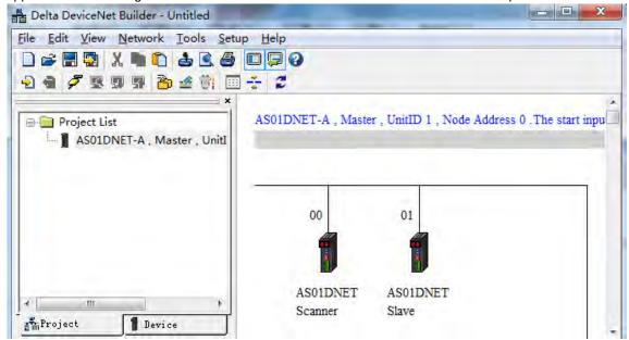
7. Double click the icon of AS01DNET Slave. Then the **Node Configuration...** dialogue box appears. Input Size and Output Size are both set to 8 bytes. Click OK to finish the setting.
