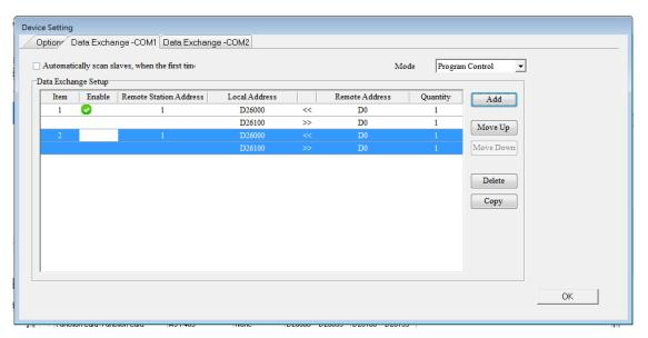
In the examples above, note that the Normal Exchange Area shows the corresponding data registers of the module and the PLC.
