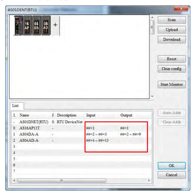
After AS01DNET (RTU) is pulled into **Scan List**, the mapping addresses that the master assigns to AS01DNET (RTU) are shown as below.
