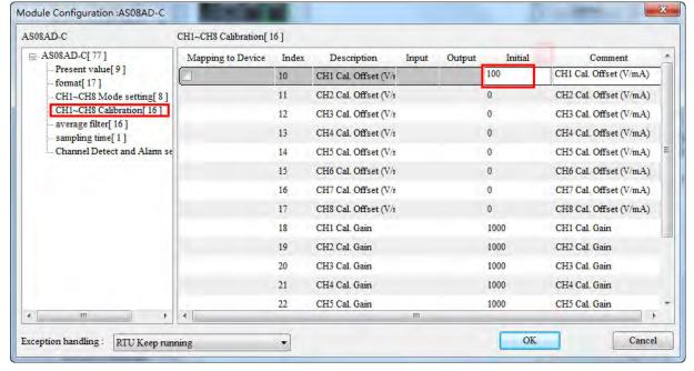
Case 3: For the module parameter which need be monitored in real time or need be modified in its value, tick the desired parameter in the **Mapping to Device** column and then the corresponding value of the parameter will map to the bus data for exchange i.e. the D registers in PLC. After the values of the ticked parameters in the **Mapping to Device** column go to the software monitor page, the current values of parameters can be monitored and modified in real time.
