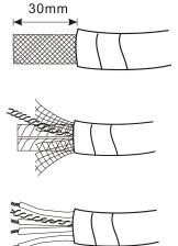
Insert the peeled communication cables into the holes in the connector in correct order.
