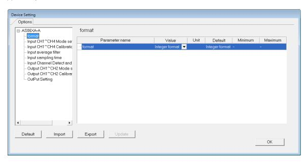
(2) Input CH1-CH4 (channel 1-channel 4) mode settings
