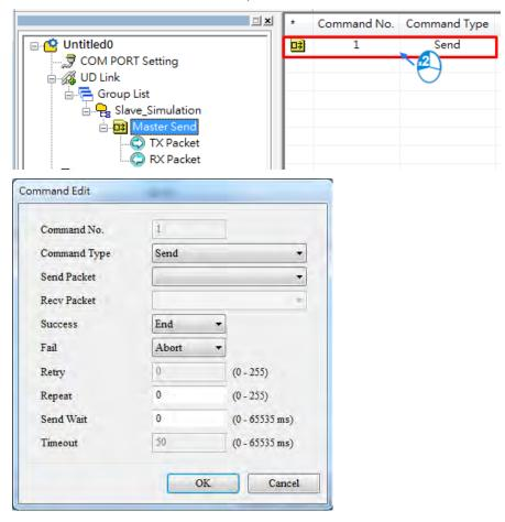
23) Set Send Packet to "TX POS Send" and set Recv Packet (received contents) to "RX Result".
