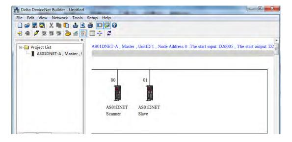
6. Click **Network** >> **Scanner Setting**. The **Scanner Setting** dialog box appears. Select **Enable** under **Extension Baudrate** and the desired baud rate as below. Click **OK** after the setting is finished.
