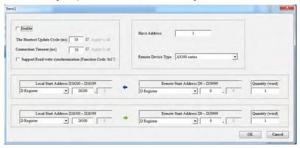
• Select **Standard Modbus Device** as the **Remote Device Type**, enter the parameters, and check **Enable**.
