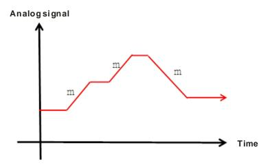
\*The output conversion time and the input channel sampling cycle are the same.
