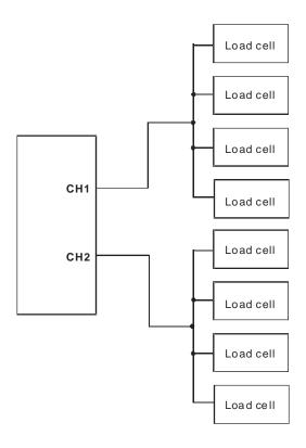
Note 1: Please connect on the power supply module and on the load cell module to a system ground, and then ground the system ground or connect the system ground to a distribution box.
