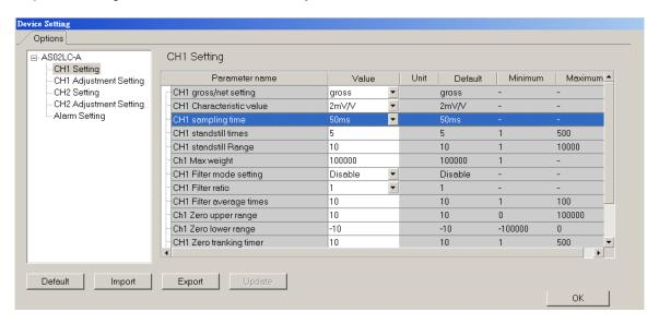
Step 2: set the number of adjustments and their corresponding values. The example below shows a 2-point adjustment where point 1 = 0 and point 2 = 1000, corresponding to 1 kg.
