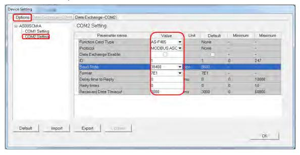
6) Set up the data exchange table: select **Data Exchange – COM2** and click **Add** to create a new Data Exchange Setup table.
