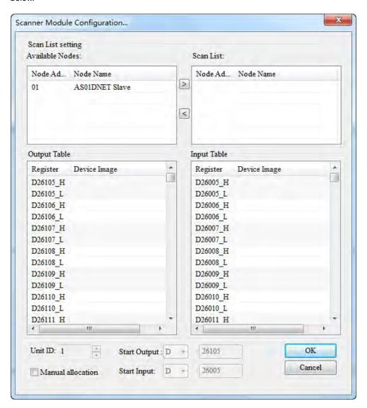
2. Move the DeviceNet slaves from the left list to Scan List of the right side. Follows the steps: Select one DeviceNet slave node and then click. Then the DeviceNet slave nodes are moved to the Scan List one by one
