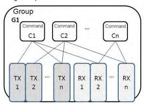
First, create TX and RX packets in a group. Then, set the sequence for sending and receiving the packets, as well as the number of times the packets are sent and received. Finally, start sending and receiving the packets in the group. If several different types of packets are required in a larger system, you can also arrange several groups in sequence and set the sequence of sending/receiving the packets in each group.
