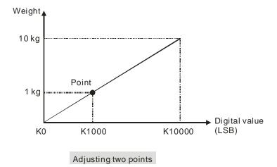
In addition to this two-point adjustment, the load cell also supports adjustments of up to 20 points. A characteristic curve is shown below.
