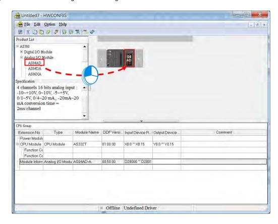
(3) Double-click the module in the working area to open the Device Setting page.
