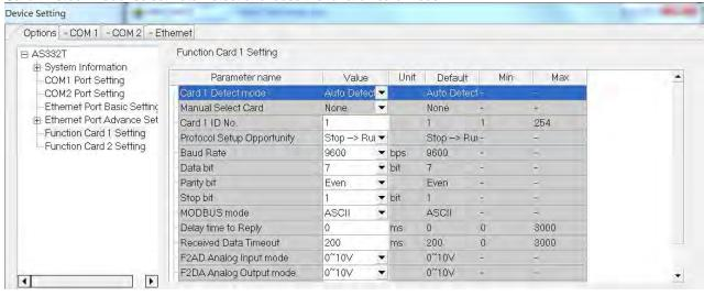
(a) When the function card is an AS-F232, AS-F422, or AS-F485, configure the communication settings in the red box.
