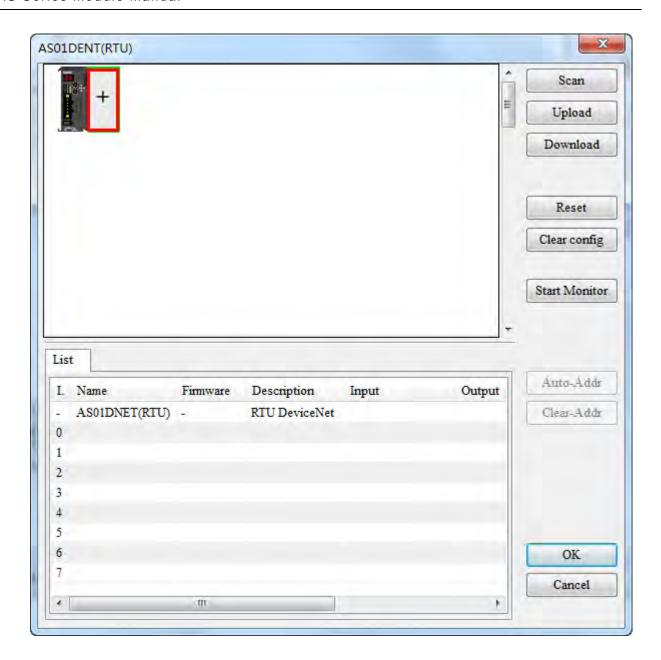
7. Click the **Scan** button to scan the I/O modules connected to the right side of AS01DNET (RTU).
