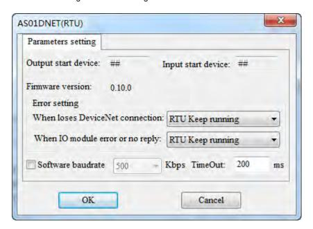
Explanation of AS01DNET (RTU) parameter setup:
