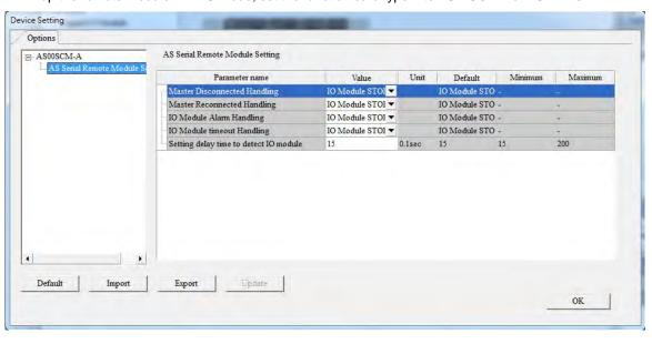
For the following four situations, you can either stop I/O module (all I/O modules stop running) or keep I/O module running (all I/O modules keep the same state).
