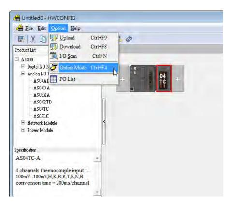
(2) Double-click the module to open the Device Setting page. The versions of both the firmware and the hardware are displayed.
