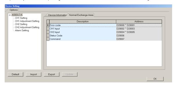
Step 6: put no load on the load cell (adjustment point 1) and enter 1 into D28007. 1 represents channel 1 and 2 represents channel 2.
