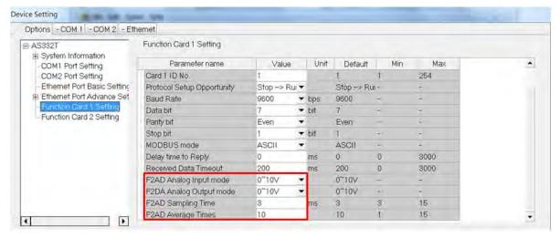
(e) When the function card is an AS-FEN02, configure the communication settings in the red box.
