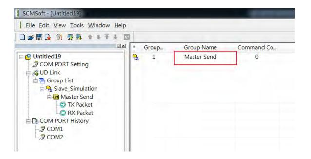
10) Right-click TX Packet and click TX Packet to create a TX Packet1.
