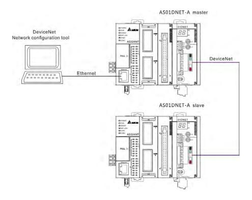
**Note**: Both of the ends of the DeviceNet Bus cable must connect one  $121\Omega$  terminal resistor respectively. The terminal resistor is connected between CAN\_H and CAN\_L.
