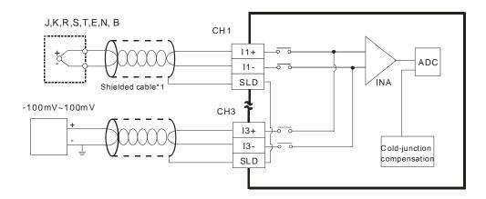
\*1. Use shielded twisted pair cables for Type J, type K, type R, type S, type T, type E, type N and type B thermocouples, and keep them separate from power cables and other cables which generate noise.
