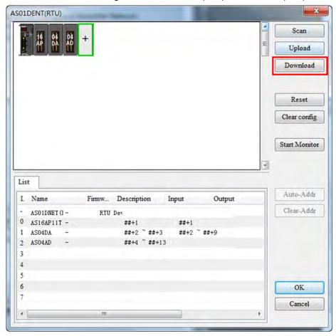
10. After the download, click the OK button to go back to the main page of the software. Double click AS01DNETScanner icon and then move the slave in Available Nodes to Scan List on the Scanner Module Configuration dialog box. Click the OK button to finish the setting.
