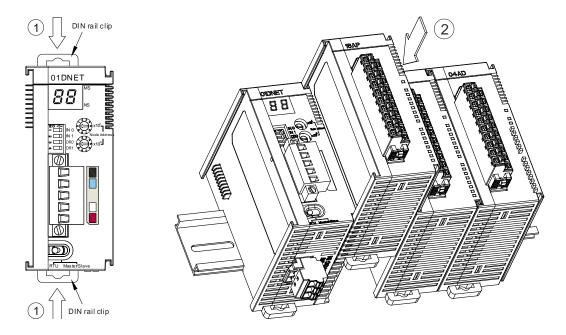
Tighten the screws on the top of the module at the end of installing.
