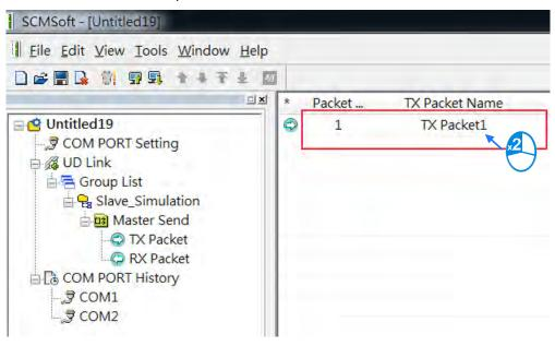
12) Give the Packet a Name (This example uses "TX POS Send")
