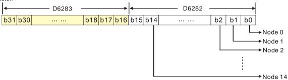
In the bit-strobe method, the master does not send control data to the slave node. However, the slave node need return I/O data to the master if the corresponding bit is set to 0. If the corresponding bit is set to 1, the slave node does not need to return I/O data to the master.
