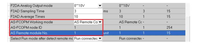
Turn the FORMAT1 switch to 0, and the adjustable range for station knob ID2 becomes 0x1h–0xFh. In AS Remote Communication mode, an AS series CPU PLC can connect to as many as 15 AS00SCM-A modules, as long as they are all in RTU mode. The RTU station number should be set from 1 to 15 in numerical order.
