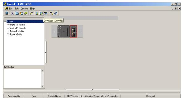
Step 3: after the configuration is complete, download the parameters to the module.
