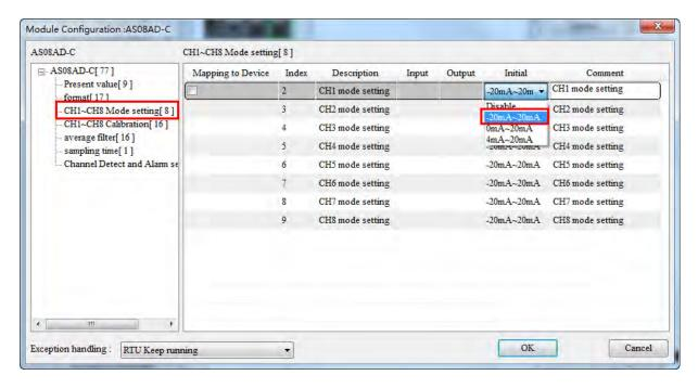
Case 2: Manually enter the value for the parameter to change in the Initial column, e.g. write 100 for CH1 Cal.Offset of AS08AD-C).
