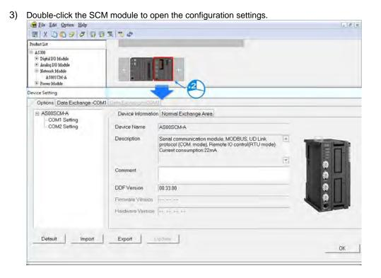
4) Set the communication protocol values for COM1 using the HMI settings.
