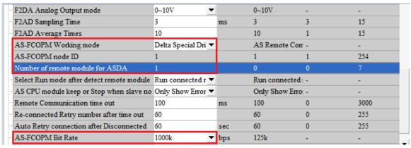
Turn the FORMAT1 switch to 8, and the adjustable range for station knob ID2 becomes 0x9h–0xFh. In the Delta Special Driver & AS Remote Mode, an AS series CPU PLC can connect to as many as 7 AS00SCM-A modules, as long as they are all in RTU mode. The RTU station number should be set from 9 to 15 in numerical order.
