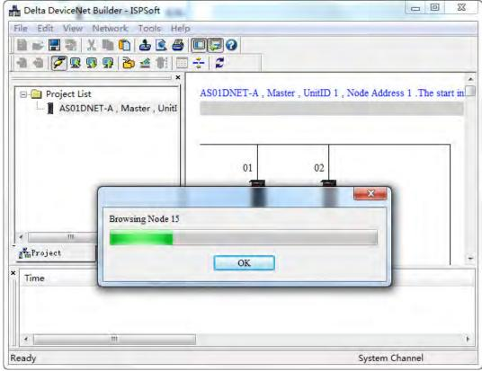
Double click AS01DNET (RTU). Then the Node Configuration... dialog box appears. Click the IO Configure... button to make the AS01RTU-DNET interface appear, where to configure the modules connected to AS01DNET (RTU).
