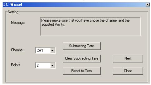
Step 6: put no load on the load cell (adjustment point 1) and click **Next** to proceed.
