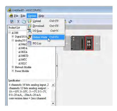
(2) Double-click the module to open the Device Setting page. The versions of both the firmware and the hardware are displayed.
