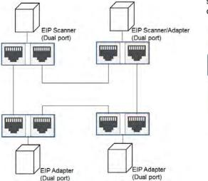
When a switch is needed for topology, the switch should support the DLR function. If not, the connection might fail
