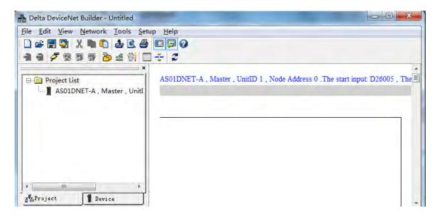
4. Clicking Network>> Scan DeviceNet Network, the DeviceNet Builder software starts to scan the whole network.
