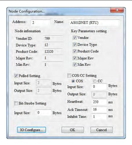
2. Click the **I/O Configure...** button in the **Node Configuration...** window. Then the main configuration page appears as below.
