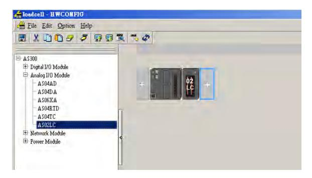
(3) Double-click the module in the working area to open the Device Setting page.
