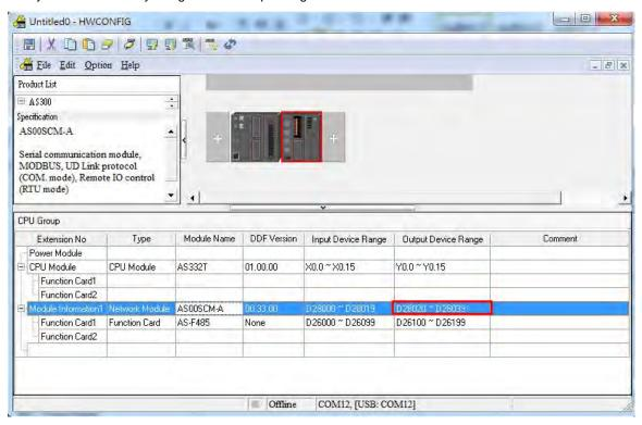
27) Double-click AS00SCM-A to open the Device Setting page. Verify that the Card 1 UD Link Group ID Trigger is set to D28030. Use ISPSoft to enter 1 into register D28030 to start the data
