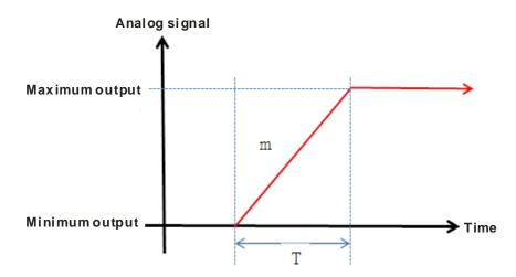
When the analog output signal changes, the system updates the value of the analog output according to the value set in the slope, as shown in the image below.
