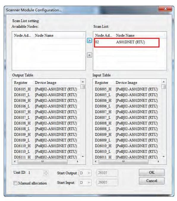
After the master assigns mapping addresses to AS01DNET (RTU), the mapping devices of the modules connected to the right side of AS01DNET (RTU) are shown as below.
