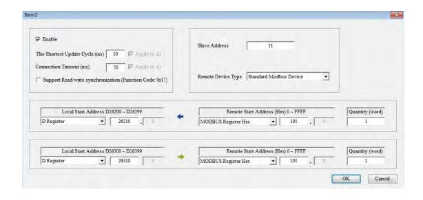
• Select **PLC devices** as the **Remote Device Type**, enter the PLC parameters, and check **Enable**.
