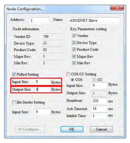
8. Right click the icon of AS01DNET Slave and click **Parameter Edit...** on the drop-down menu. The **Parameters Edit...** dialog box appears and **Polled Input Length** and **Polled Output Length** are both set to 8 bytes as shown in the following red box. Then click **Write** button. Click **OK** after writing is finished. Afterwards, repower AS01DNETSlave.
