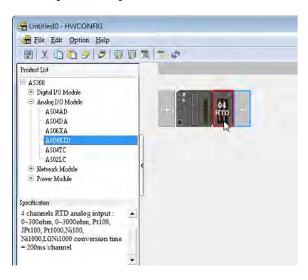
(3) Double-click the module in the working area to open the Device Setting page.
