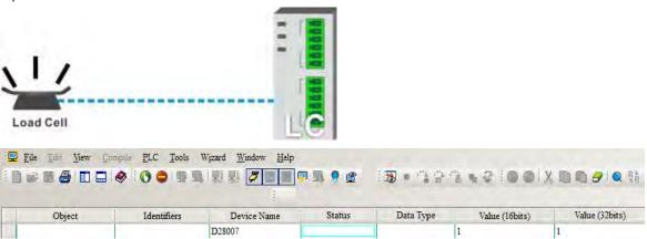
Step 7: put a load on the load cell (adjustment point 2). For multi-point adjustment, repeat this step. This example uses a 1 kg weight.
