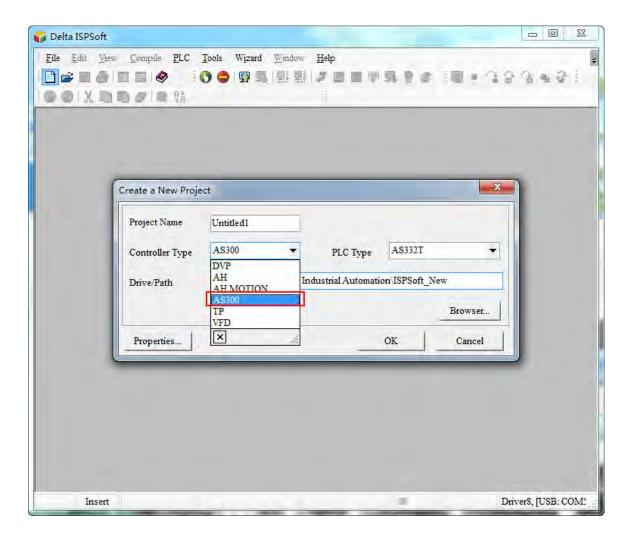
Note: The PLC type used in this section is AS332T-A.
