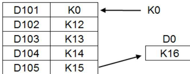
6. Execute the instruction DTM for 5 times to have the results: D0=K12 and values in D101~105 are K0.
