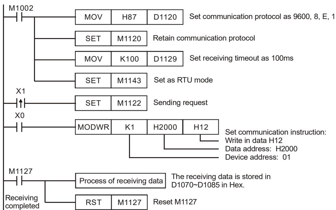
PLC → VFD-B, PLC transmits: 01 06 2000 0012 02 07
