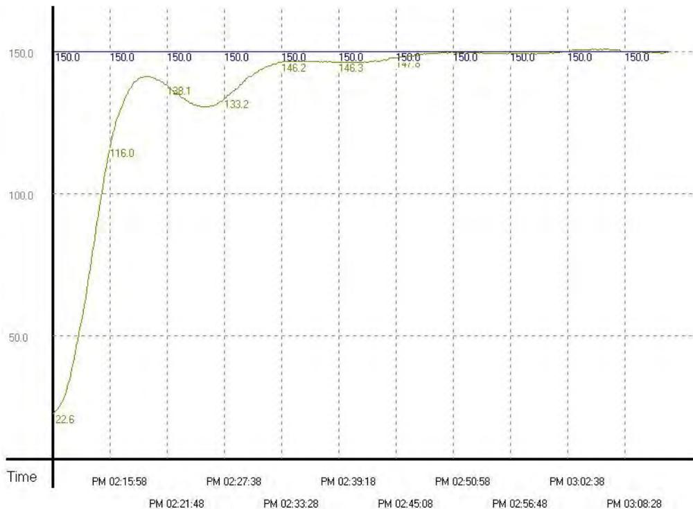
**Example 4:** To see if we can reach the target temperature faster, we modify the sampling time from example 3 into 2 seconds (D12 = K20, D30 = K2,000). The results are shown in the diagram below. From the diagram below, we see that the sampling time that is too short will cause the control system to become too sensitive and lead to up and down fluctuations.
