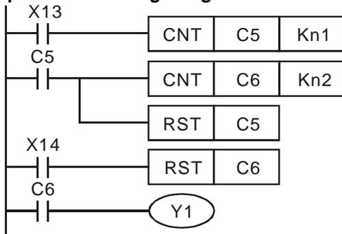
The counting range of a 16-bit counter is 0 ~ 32,767. The opposite circuit uses two counters to increase the counting range as  $n1*n2$ . When value in counter C6 reaches  $n2$ , The pulses counted from X13 will be  $n1*n2$ .
