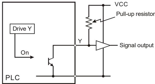
5. Positive logic (negative polarity) output of BCD code
