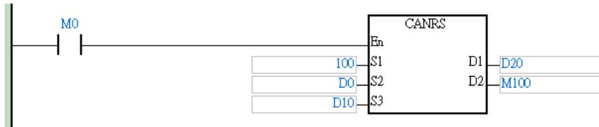
Step 5) after receiving data is complete, M100 will be ON; check if the value in D1175 is NOT 0. When there is any value in D1175 other than zero, it indicates D20 has received responses from the slaves.
