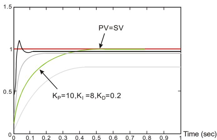
Note: The example is only for reference. Users have to adjust parameters according to the condition of the actual control system.
