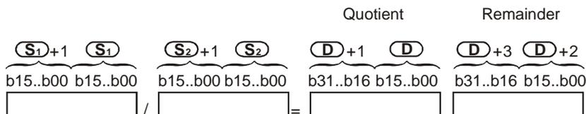
If D is specified with a bit device, it can designate K1 ~ K8 to store a 32-bit result. Users can use consecutive 2 32-bit registers to store the quotient and remainder.
