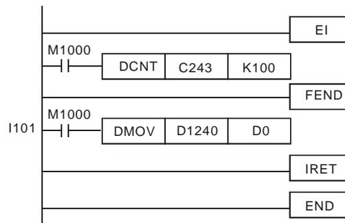
When C243 is counting and external interrupt is triggered from X1(I101), counted value in C243 will be move to (D1241, D1240) immediately then C243 is reset. After this interrupt I101 executes.
