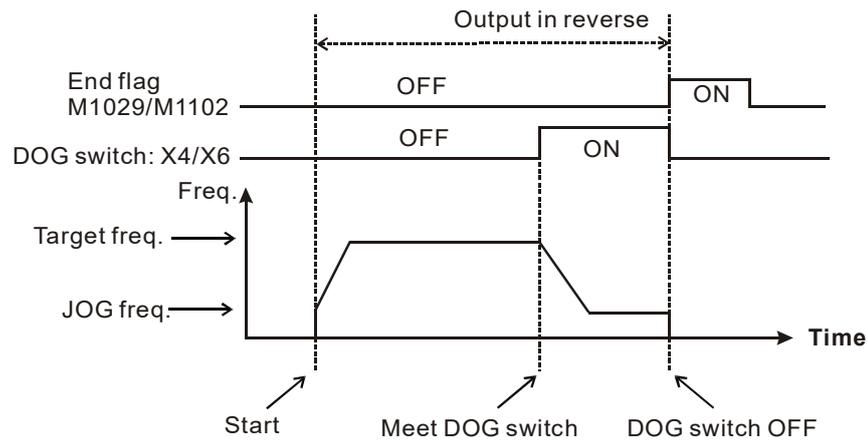
State 2: DOG switch is ON, pulse output in reverse, limit switch disabled.
