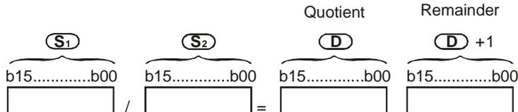
If D is specified with a bit device, it can designate K1 ~ K4 to store a 16-bit result. Users can use consecutive 2 16-bit registers to store 32-bit data of the quotient and remainder.
