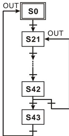
b) The control power over the step is transferred to the step in another sequence.
