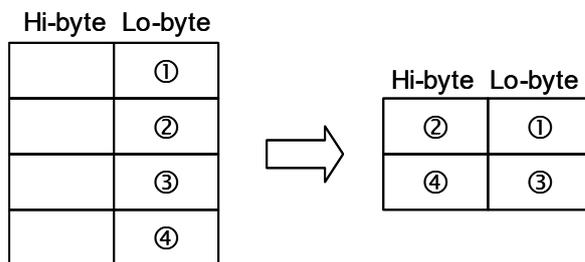
K2: With  $n = 2$ , transform 16-bit data (Hi-byte, Lo-byte) into 8-bit data in the following rule:
