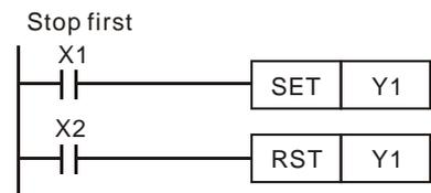
Stop First circuit while SET which is lower than RST forms a Start First circuit.
