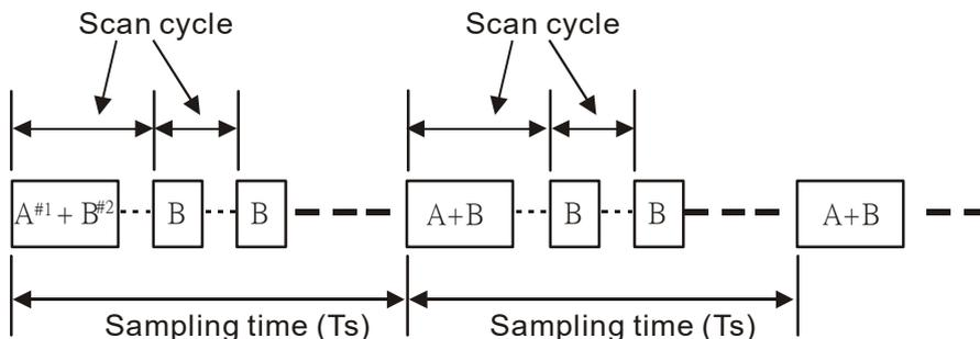
Note: #1→ The time for equation calculation during PID operation (approx. 72us)
