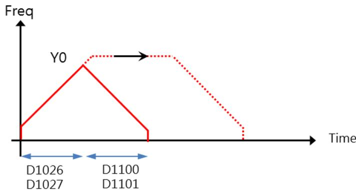
B. When the masking number is -1 in the front masking area, it indicates masking occurs in the acceleration area; -2 in the front masking area means masking occurs in the areas of acceleration and full-speed; -3 (only available for DCLLM instruction) in the front masking area means masking occurs in the areas of acceleration, full-speed and deceleration.
