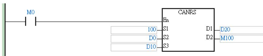
Step 6) after receiving data is complete, M100 will be ON; stop executing CANRS instruction (RST M0).
