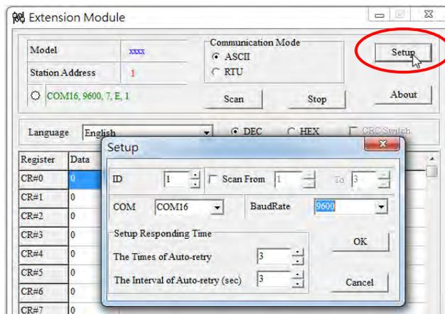
Step 3: Click **Scan** to connect to the module and monitor the current values of the control registers
