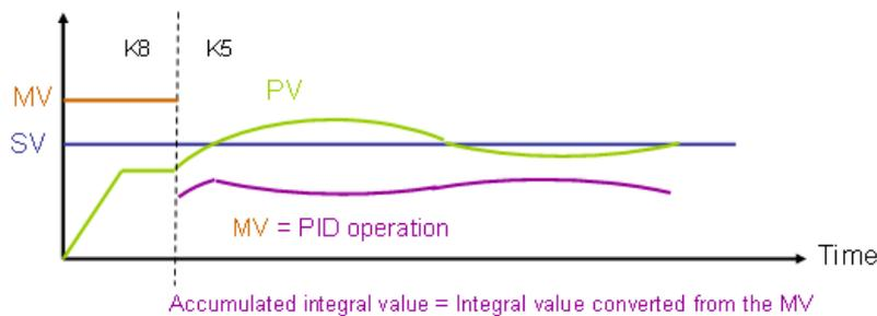
If the control mode becomes the automatic mode (K5), the accumulated integral value will be the integral value converted from the last MV, and the accumulated integral value will be converted into the output value of the PID operation.
