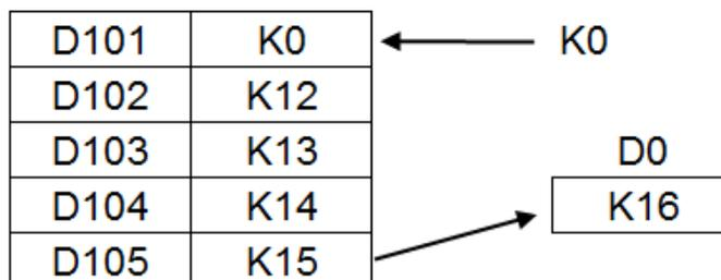
3. Execute the instruction DTM for 5 times to have the results: D0=K12 and values in D101~105 are K0.
