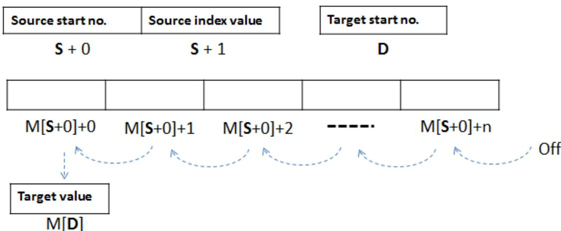
Note 1: When the value in S+1 is less than 1, it means there is no data to be read/moved and no action will be taken. When the value in S+1 is bigger than n, it means the data is full and no action will be taken. "No action will be taken" means no error will be displayed nor will the index value (S+1) have any change.
