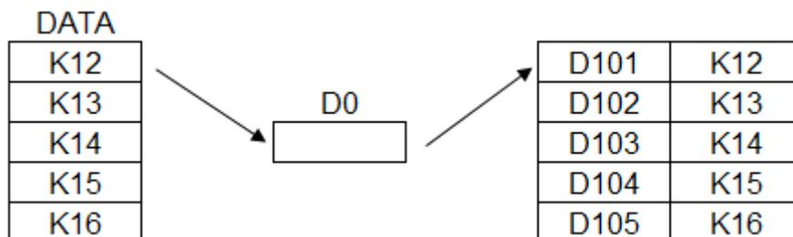
2. Adding one to the value stored in D100, after the execution of the DTM instruction is complete.
