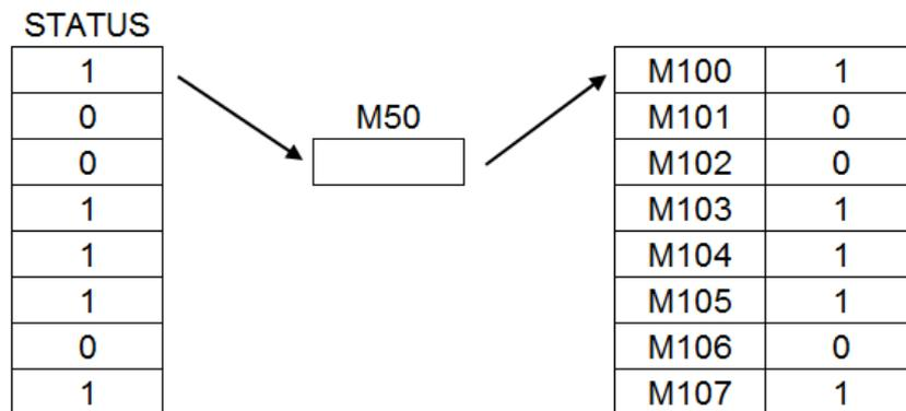
K35: Read the first written BIT data to the BIT device (target value) and move the succeeding BIT data forward, for example, move the second BIT data to where the first written BIT data was and so on. (first in first out)
