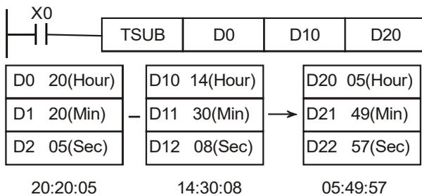
If the subtraction result is a negative value (less than 0), Borrow flag M1021 = ON.
