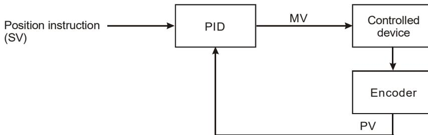
**Example 2:** Block diagram of application on AC motor drive ( $S_3+4 = 0$ )
