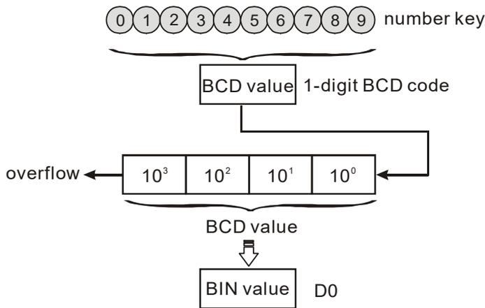
2. As shown in the timing diagram below, four keys connected with X35, X33, X31 and X30 are pressed in order. Therefore, the number 5,301 is generated and stored in D0. 9,999 is the maximum value allowed for D0. If the entered number exceeds the available range, the highest digit performs overflow.
