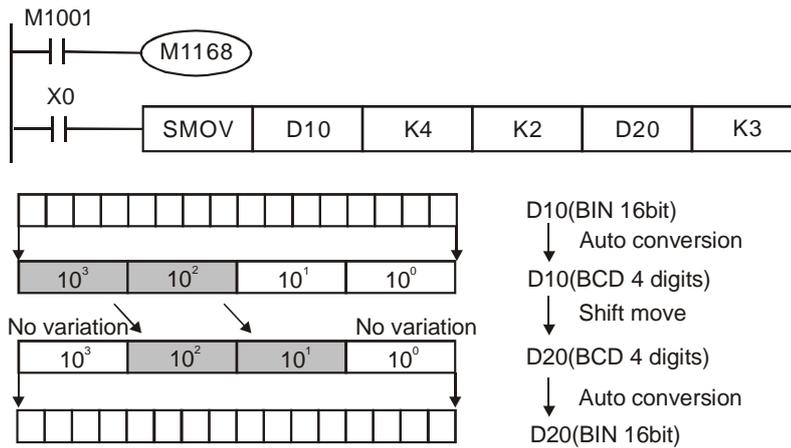
If D10 = K1234, D20 = K5678 before execution, D10 remains unchanged and D20 = K5128 after execution.
