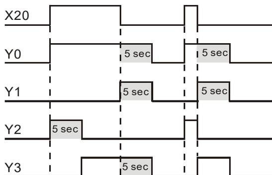
6. Apply a NC contact Y3 after the drive contact X20, and Y1, Y2 will form a flashing circuit output. When X20 turns OFF, Y0, Y1 and Y3 = OFF and the content of T10 will be reset.
