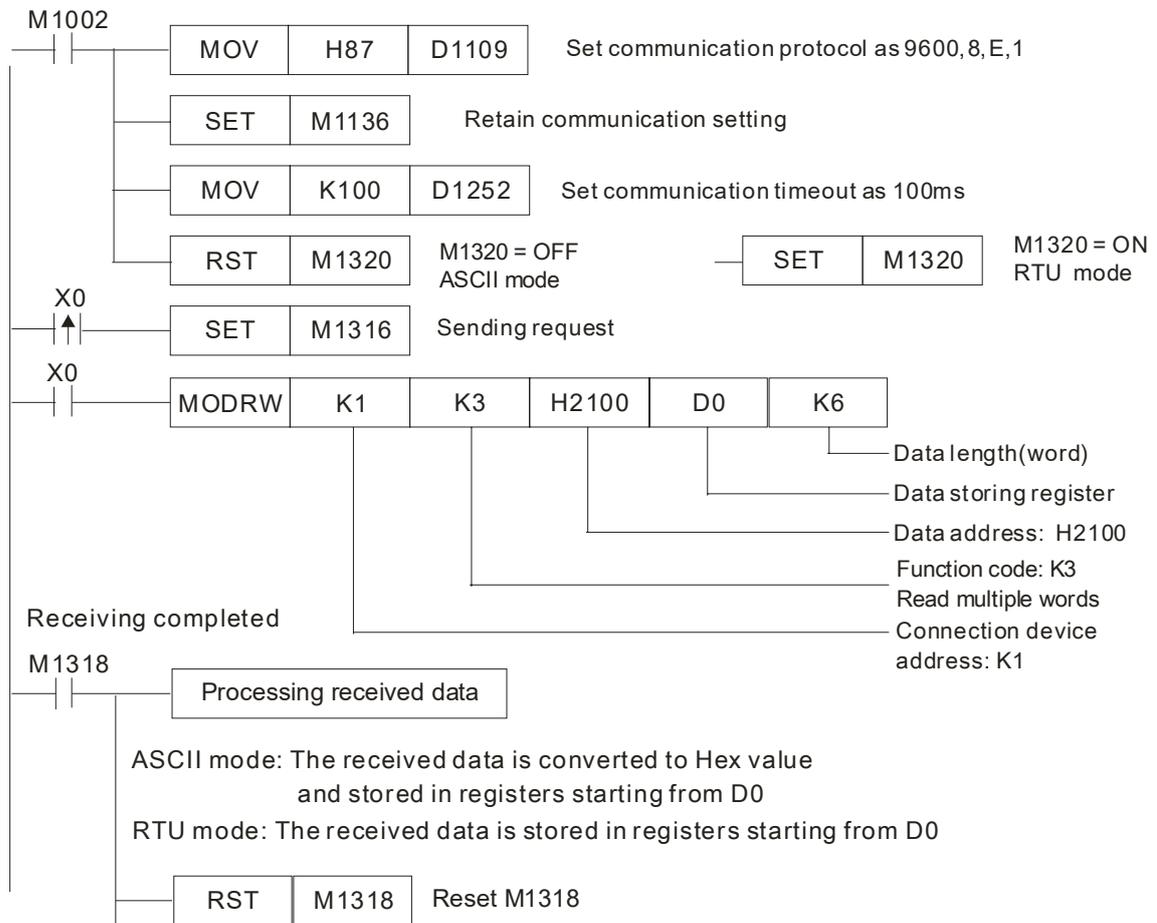
**ASCII mode (COM3: M1320 = OFF, COM1: M1139 = OFF):**
