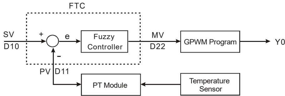
Output D22 (MV) of FTC instruction is the input D22 of GPWM instruction, as the duty cycle of adjustable pulses. D30 is the fixed cycle time of pulses. See below for the timing diagram of Y0 output.
