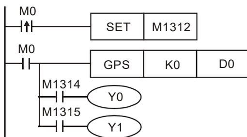
3. When receiving completed, M1314 = ON. When receiving failed, M1315 = ON. The received data will be stored in devices starting with D0.
