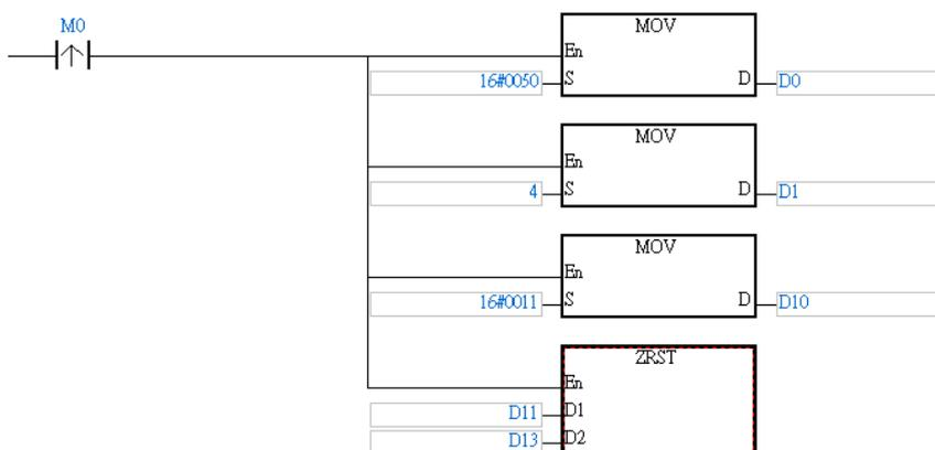
Step 4) LD M0 → use CANRS instruction to set the first left-side module COPM-SL to send data
