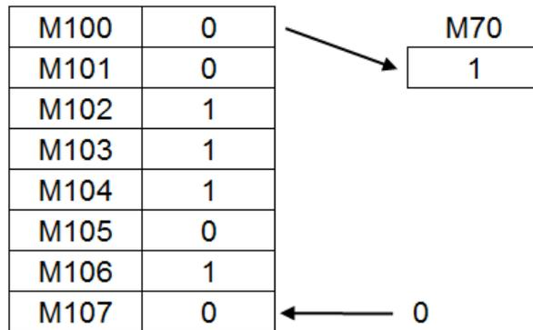
3. Execute the instruction DTM for 8 times to have the results: M70=1 and the states in M100~M107 are 0.
