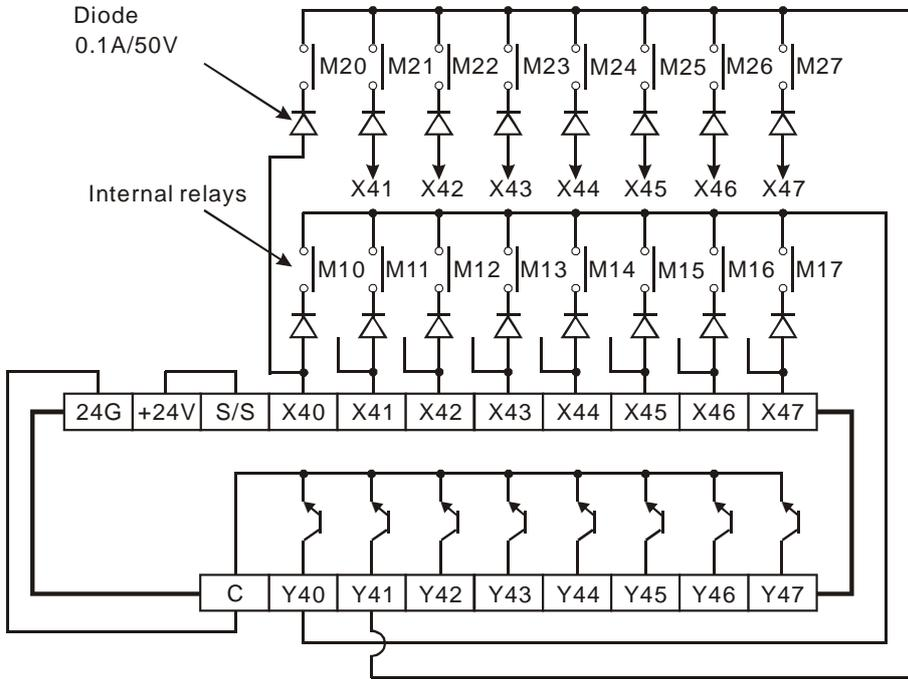
When output Y40 is ON, only inputs in the first array are read. The results are stored in auxiliary relays M10~M17. After Y40 goes OFF, Y41 turns ON. This time only inputs in the second array are read. The results are stored in M20~M27.
