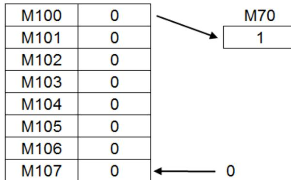
K36: Read the last written register to the D device (target value) (last in first out).
