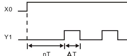
When X0 = ON, T0 starts timing ( $nT$ ). Once the set time is reached, contact T0 = ON to enable Y1( $\Delta T$ ). In next scan, Timer T0 is reset due to the reversed status of contact Y1. Therefore contact T0 is reset and Y1 = OFF. In next scan, T0 starts timing again. The process forms an oscillating circuit with output cycle  $nT + \Delta T$ .
