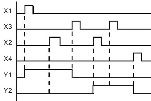
NC contact Y1 is connected to Y2 output circuit and NC contact Y2 is connected Y1 output circuit. If Y1 is ON, Y2 will definitely be OFF and vice versa. This forms an Interlock circuit which prevents both outputs to be ON at the same time. Even if both X1 and X2 are ON, in this case only Y1 will be enabled.
