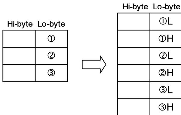
K6: When n = 4, transform 8-bit ASCII data (higher 4 bits, lower 4 bits) into HEX data in the following rule: (ASCII value to be transformed includes 0 ~ 9 (0x30~0x39), A ~ F (0x41~0x46), and a ~ f (0x61~0x66).)
