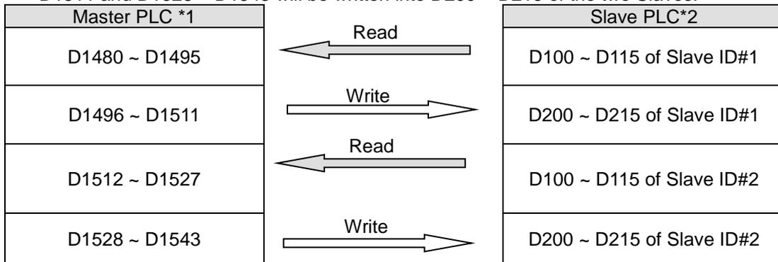
c) Assume the data in registers for data exchange before enabling PLC LINK (M1350 = OFF) is as below:
