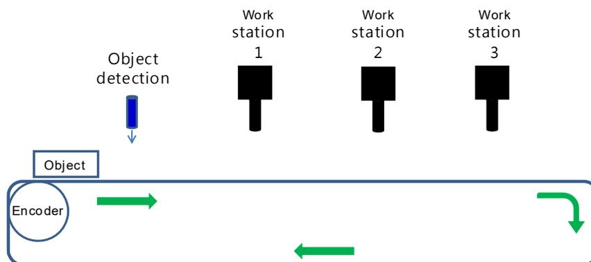
**Step 1:** use the input point X4 as the object detection interrupt, C251 as the high-speed counter for the encoder and output point Y0 as the first output point for the work station.
