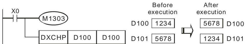
4. When X0 = ON and M1303 = ON, the high 8 bits and the low 8 bits in D0 are exchanged, the high 8 bits and the low 8 bits in D1 are exchanged., and the high 8 bits and the low 8 bits in D2 are exchanged.
