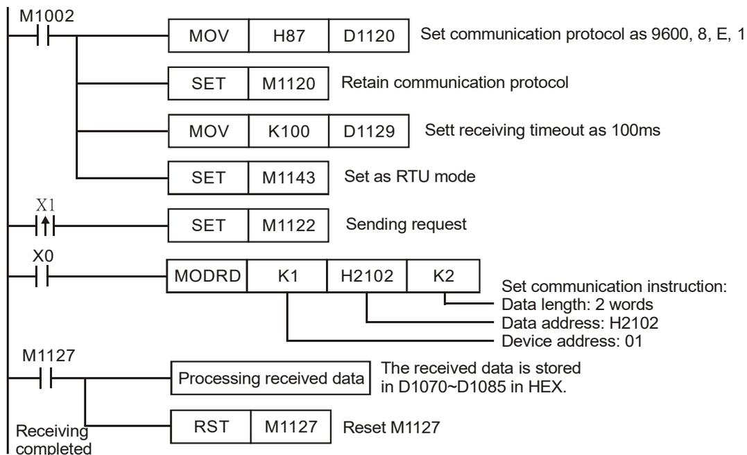
PLC → VFD-B , PLC transmits: 01 03 2102 0002 6F F7
