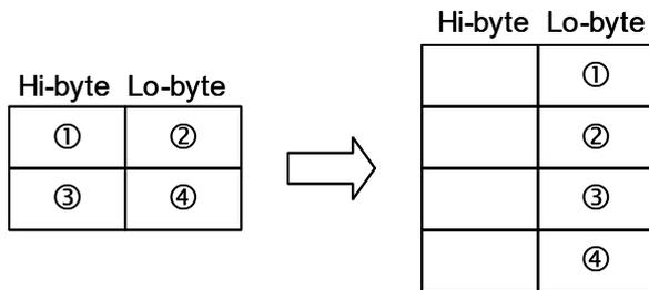
K3: With  $n = 2$ , transform 16-bit data (Lo-byte, Hi-byte) into 8-bit data in the following rule:
