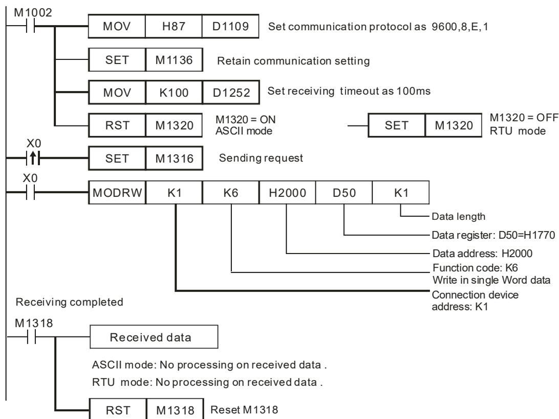
**ASCII mode (COM3: M1320 = OFF, COM1: M1139 = OFF):**
