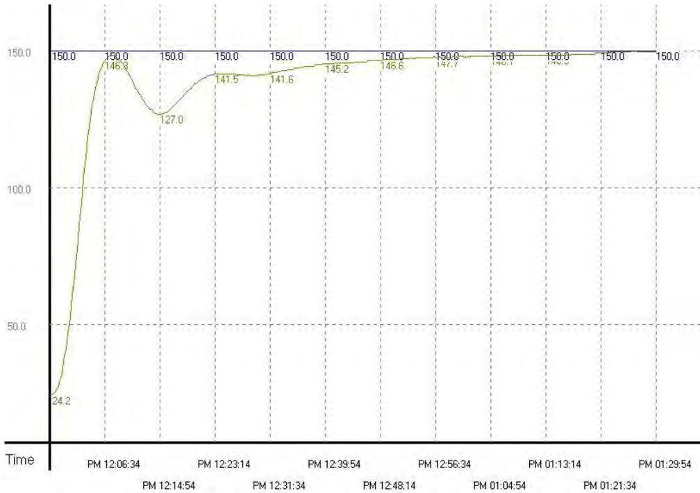
**Example 3:** To speed up the speed to reach the target temperature, we correct the sampling time as 4 seconds (D12 = K40, D30 = K4,000). The results are shown in the diagram below. From the diagram below, we see that the overall control time has been shortened as 37 minutes. Therefore, we find out that modifying the sampling time can speed up the time for reaching the target temperature.
