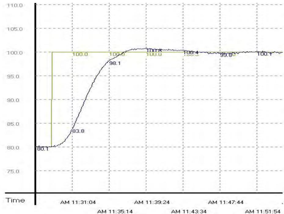
From the result above, we can see that when the parameter is 100°C, temperature control works fine and costs only 20 minutes same as that in 80°C.
