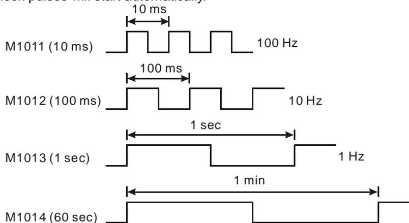
2. Clock pulse works even when PLC stops, i.e. activation of clock pulse is not synchronized with PLC RUN execution.
