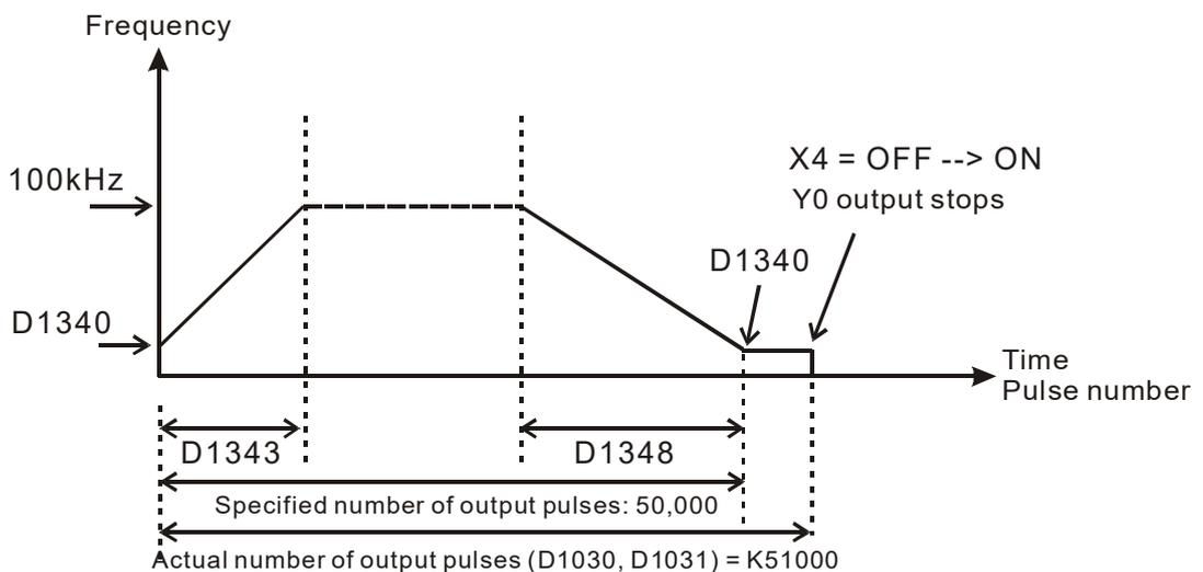
**Program Example 2:** Immediate stop high-speed pulse output by high speed counter
