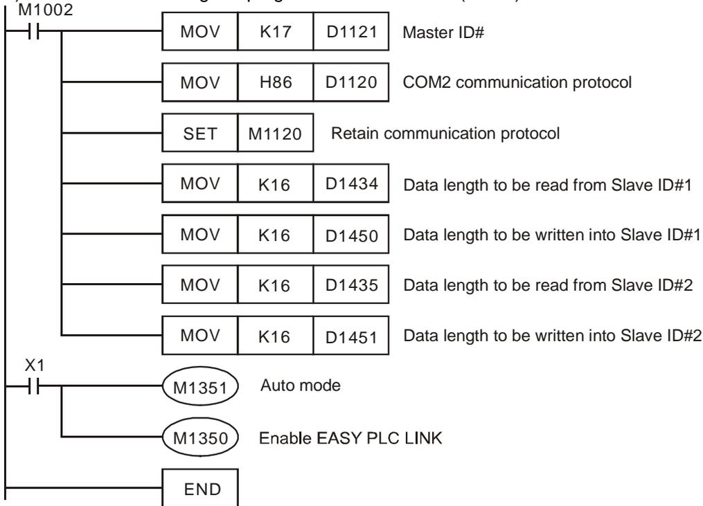
b) When X1 = On, the data exchange between Master and the two Slaves will be automatically executed by PLC LINK. The data in D100 ~ D115 in the two Slaves will be read into D1480 ~ D1495 and D1512 ~ D1527 of the Master, and the data in D1496 ~ D1511 and D1528 ~ D1543 will be written into D200 ~ D215 of the two Slaves.
