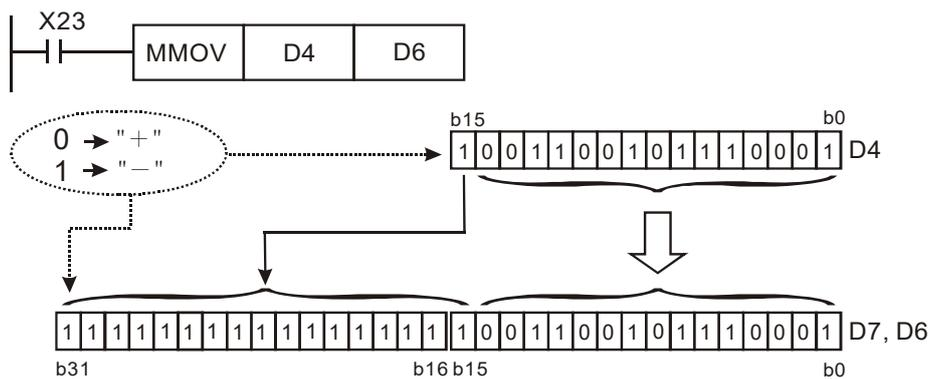
In the example above, b15 in D4 will be sent to b15~b31 of D7/D6, therefore all bits in b15~b31 will be "negative."
