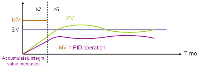
If the control mode becomes the automatic mode (K5), the output value MV changes from the output value set by users to the output value of the PID operation.
