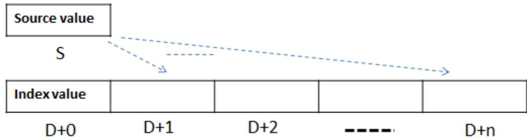
Note1: when the index value (D+0) is less than 1, it will be treated as 1 and the actions of data copy and accumulation begin. When the index value (D+0) is bigger than n (default: n+1), the action of data copy will not begin.
