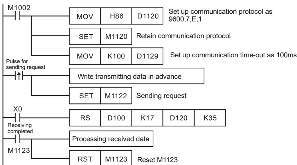
PLC ⇒ VFD-B, PLC sends “: 01 03 2101 0006 D4 CR LF “
