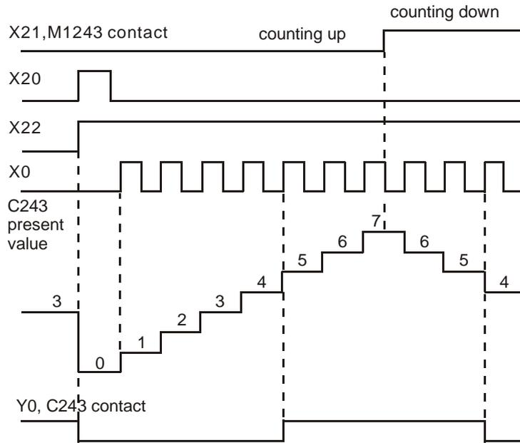
**1-phase 2 inputs high-speed counter:**
