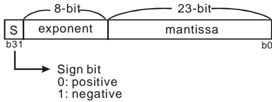
$$\text{Equation } (-1)^S \times 2^{E-B} \times 1.M; B = 127$$
