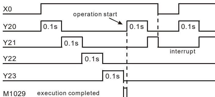
3. Please use transistor output for Y20 ~ Y23. Every pin 1, 2, 4, 8 shall be connected to a diode (0.1A/50V) in series before connecting to the input terminals on PLC.
