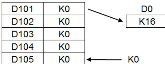
K33: Read the last written register to the D device (target value) (last in first out).
