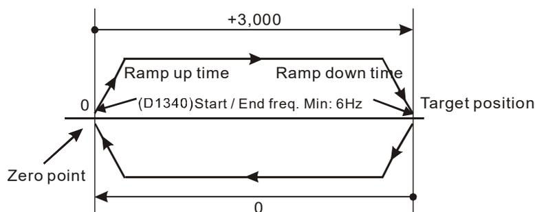
2. Registers for setting ramp up/down time and start/end frequency:
