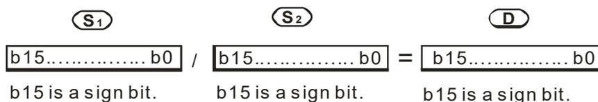
If  $D$  is a bit device, users can use K1~K4, and form 16 bits.  $D$  only occupies 16 bits.
