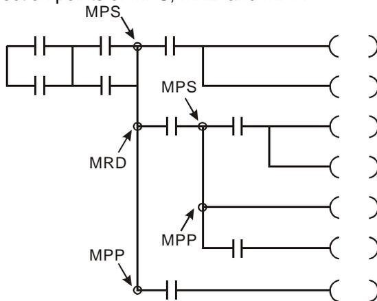
Note: Ladder diagram editor in ISPSOft does not support MPS, MRD and MPP instructions. To achieve the same results as branch instructions, users have to connect all branches to the left hand bus bar.
