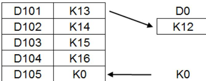
3. Execute the instruction DTM for 5 times to have the results: D0=K16 and values in D101~105 are K0.
