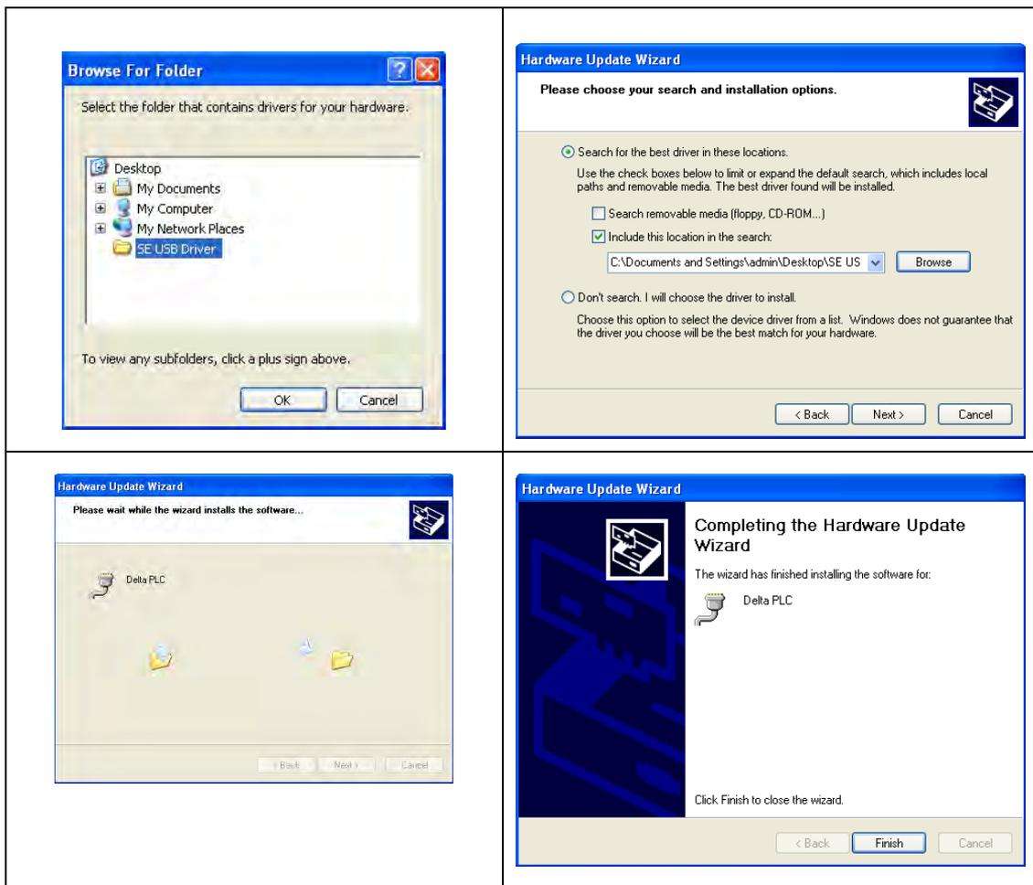
After the driver is installed, users can find the **Delta PLC** device and the communication port assigned to it in the **Device Manger** window. The usage of this device is the same as that of RS-232.
