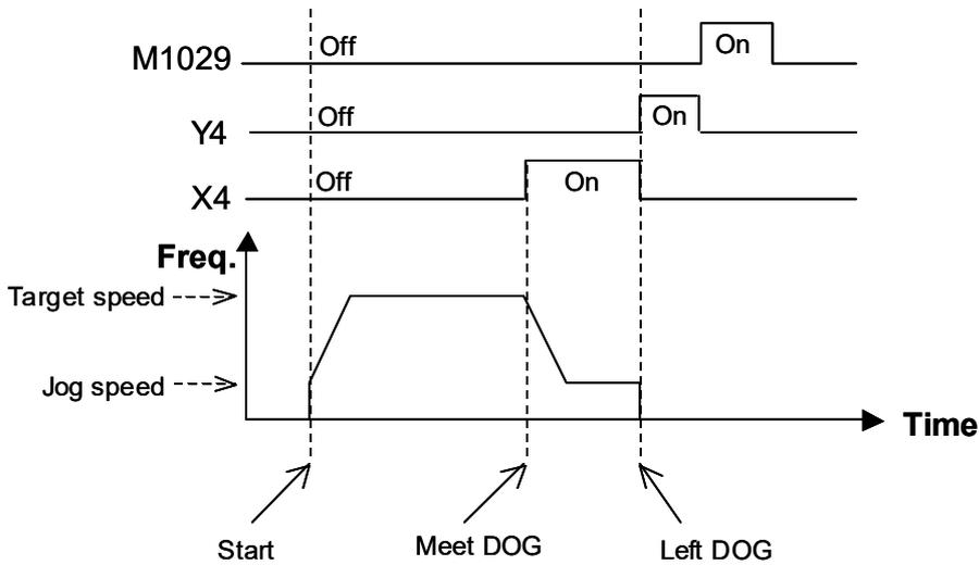
State 5: Current position at right side of zero point, D1312=-2, M1308=Off, M1346=On.
