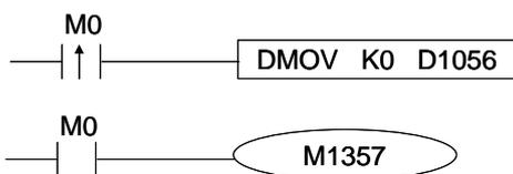
If X0's input frequency is 50Hz, the 32-bit value in (D1057, D1056) will be K50000.
