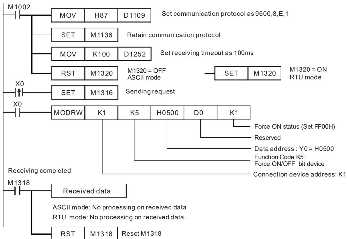
**ASCII mode (COM3: M1320 = OFF, COM1: M1139 = OFF):**
