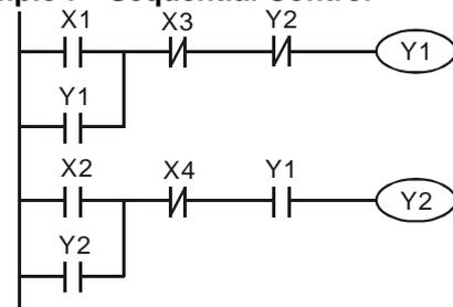
Connect NC contact Y2 to Y1 output circuit and NO contact Y1 to Y2 output circuit. Y1 becomes one of the conditions to turn on Y2. In addition, Y1 will be OFF when Y2 is ON, which forms an sequential control process.
