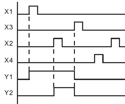
Because NO contact Y1 is connected to the circuit of Y2 output, Y1 becomes one of the conditions for enabling Y2, i.e. for turning on Y2, Y1 has to be ON
