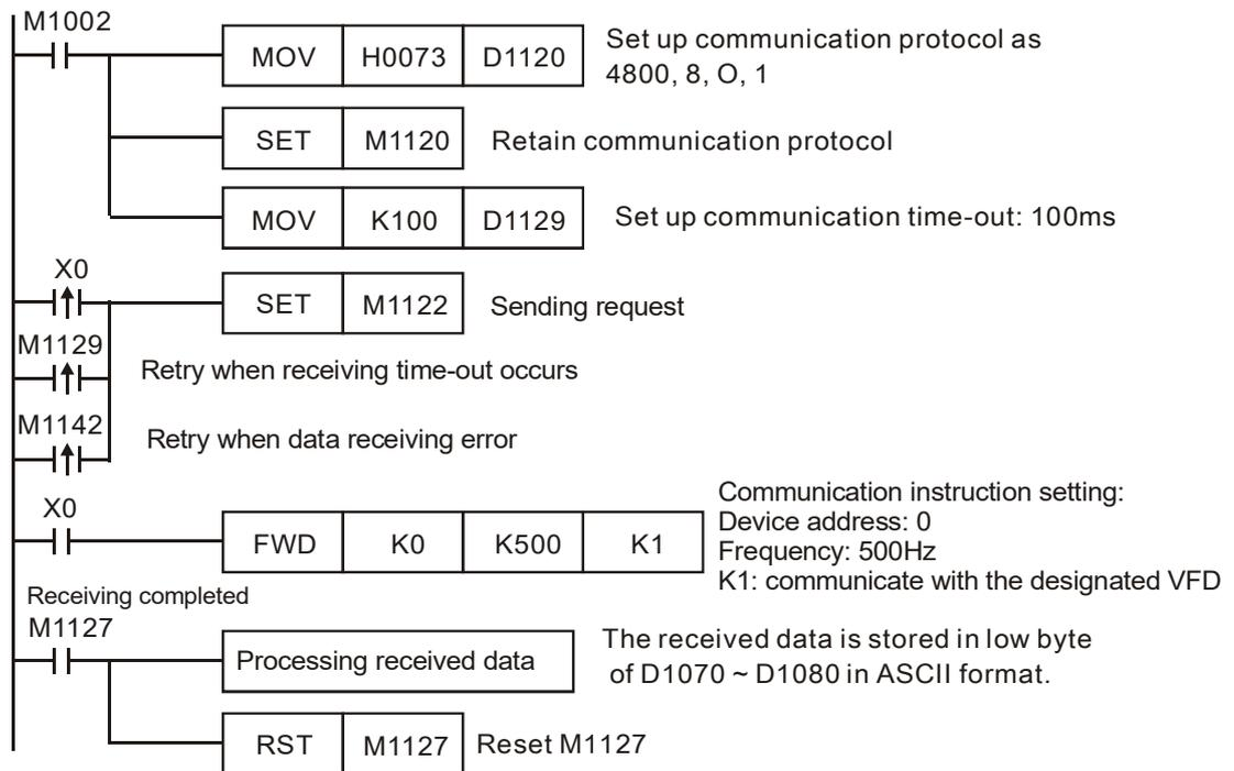
PLC ⇔ VFD-A, PLC sends: "C ♥ ☺ 0001 0500 "
