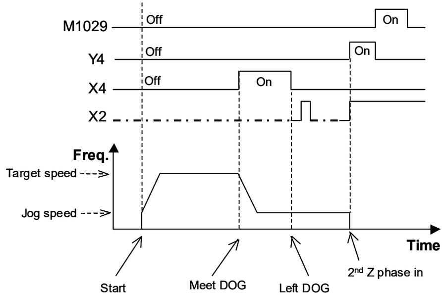
State 6: Current position at right side of zero point, D1312=-100, M1308=On.
