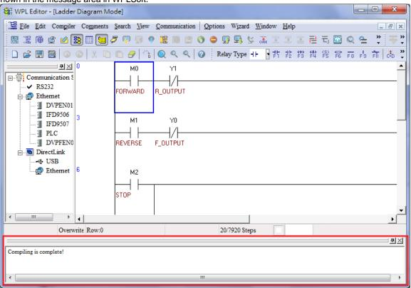
After the program is compiled, the users can download the program. After the users click **Setup** window will appear. The users can select checkboxes in the **Transfer Setup** window. Owing to the fact that there are comments on the devices in the program, the **Device Comment** checkbox in the **Transfer Setup** window is selected.
