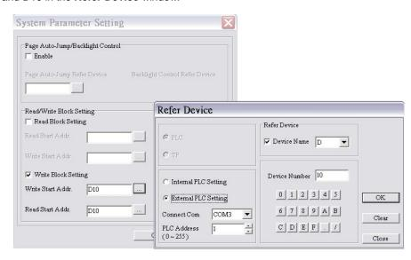
**Step 3:** After the steps above are complete, and the program in TPEditor is downloaded to TP70P, TP70P can exchange data with the DVP PLC series by means of COM3.
