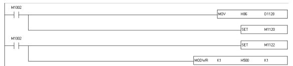
**Step 2:** Connect COM2 to the two RS-485 wires connected to a DVP series PLC. When TP70P runs, Y0 on the DVP series PLC is ON.
