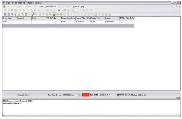
The error code shown in the figure above is HD03. It indicates that the operands of the instruction DHSCS are invalid. After DHSCS is checked, and the operands are modified, the error will be eliminated.
