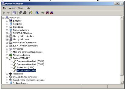
The communication port which is connected to TP70P is also shown in the PC COM Port box in the PC Communication Setting (PC <=> TP) section in TPEditor.
