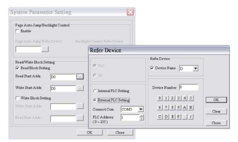
• Write Block Setting: The values in D10~D17 in TP70P are written to D10~D17 in the DVP series PLC.
