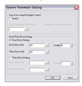
Step 3: Click .... at the right side of the Read Start Addr. box. Select the External PLC Setting option button and D0 in the Refer Device window.
