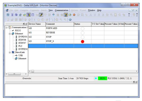
The states of the devices broght into the device monitoring table will be shown only if [ is pressed. If the users want to chage the state of a device, they can right-click the device, and click an item on the context menu which appears. M0 is set to ON here. When M0 is ON, Y0 is ON, the AC motor drive used rotates forwards, and the users can see that the forward rotation indicator on the screen of TP70P is green.
