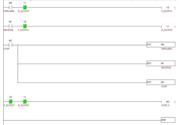
If the users want to chage the state of a device, they can right-click the device, and click an item on the context menu which appears. In the figure below, M0 is set to ON.
