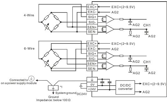
\*1. Connect the  $\stackrel{\perp}{=}$  of a power supply module and the  $\stackrel{\perp}{=}$  of the load cell terminal FE to the system ground and then ground the system ground or connect the system ground to a distribution box
