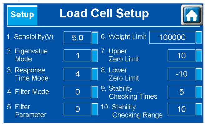
(1) Sensibility (V): set up the excitation voltage at the load cell, ranging from 2.0 V to 9.5 V.
