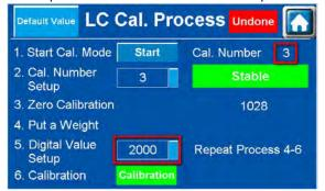
(7) After all calibrations are complete, the LC Cal. Process condition shown in the upper right corner changes from Undone in a red block to Done in a green block. Press Storing Data in the lower right corner to save the settings. Otherwise, the changes will not be saved. Press Default Value in the upper left corner to cancel without saving the changes. You can always reset calibrations to default settings by pressing Default Value in the upper left corner.
