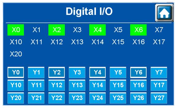
TP70P-211LC1T is with 17 digital inputs and 24 digital outputs. When an input point detects a signal, its corresponding input point in the bulletin is highlighted in a green block. The output points Y0-Y27 can be pressed to send signal to its corresponding devices. The example image shown above uses Y0, Y2, Y4, and Y6 to send signals and once X0, X2, X4 and X6 detect signals, the corresponding input points in the bulletin are highlighted in green blocks.
