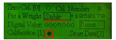
(7) After all calibrations are complete, the **Undone** changes to **Done** and **Store Data [2]** is shown in the lower right corner, as the image shown below. Press to save the settings. Otherwise, the changes will not be saved.
