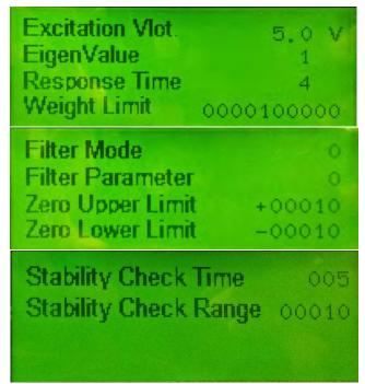
(1) Excitation Voltage: set up the excitation voltage at the load cell, ranging from 2.0 V to 9.5 V.
