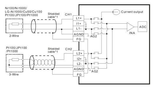
\*1. Use shielded cables to isolate the analog input signal cable from other power cables.
