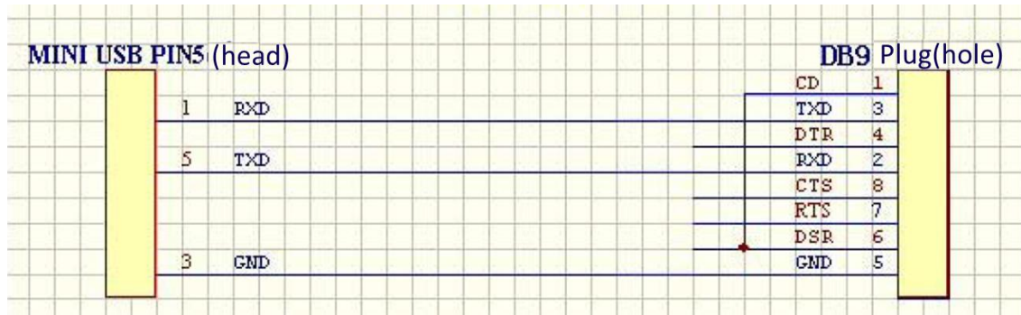
Figure3-4 Cable connection at the console port
