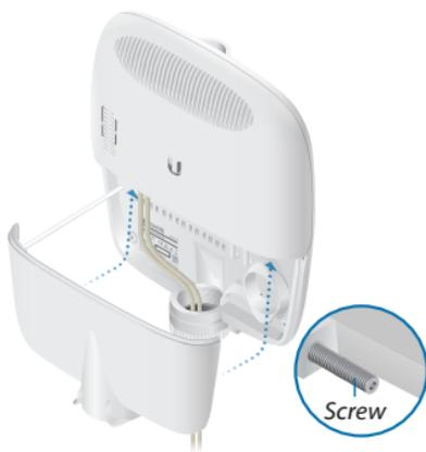
3. Wire the other end of the cable to a DC power supply.
