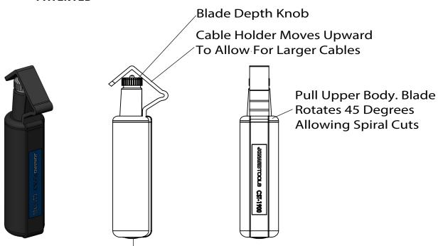
Rotate Body 90 Degrees For Longitudinal Cuts
