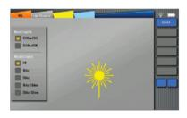
Invisible light source (1310 or 1550ns) can provide the following types of light, including CW light, 1kHz light, 2kHz light, 1kHz blink light, 2kHz blink light.
